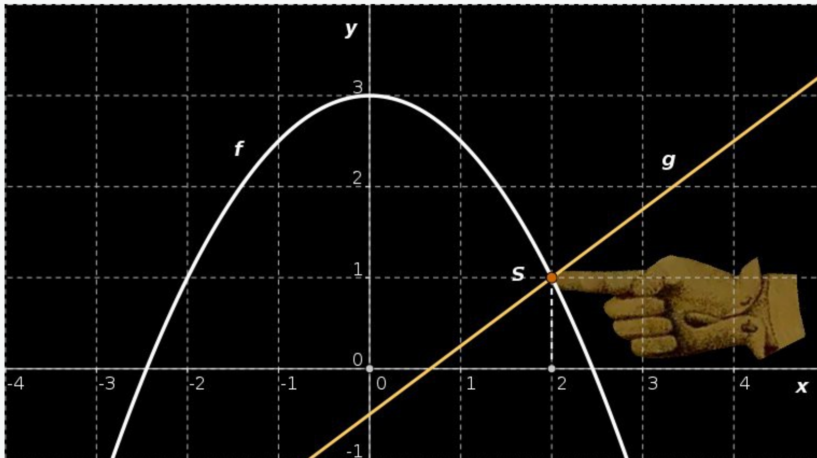
Fig. 1-2: The quadratic function y = f(x) and linear function y = g(x) have one intersection S in the positive domain
